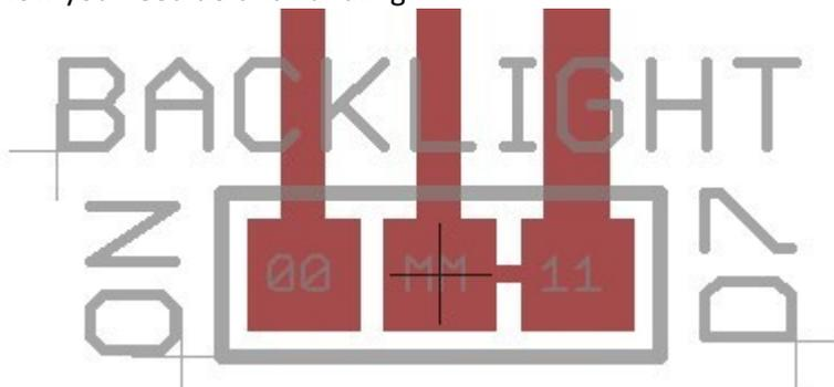
Disconnect the connection with ON pin, and connect the backlight pin with D7 pin. Of course, controlling its state is as simple as controlling a LED.
