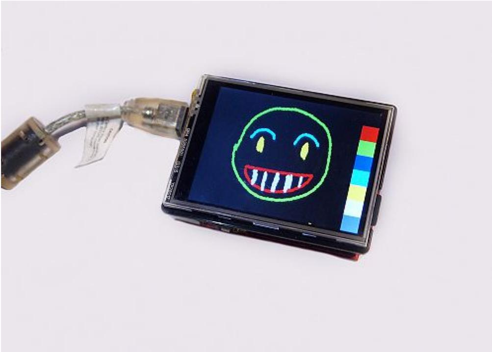
4. If you want to start painting patterns, simply press the reset button or power off and then power-on the Shield.
