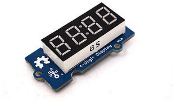
Grove - 4-Digit Display module is a 12-pin module. In this module, we utilize a TM1637 to scale down the number of controlling pins to 2. That is to say, it controls both the content and the luminance via only 2 digital pins of Arduino or Seedeuino. For projects that require alpha-numeric display, this can be a nice choice.
