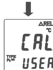
**⚠** Insert temperature probe into 0°C Deg. Standard calibration unit before calibration. Hold the probe until condition is stabilized before starting calibration.
