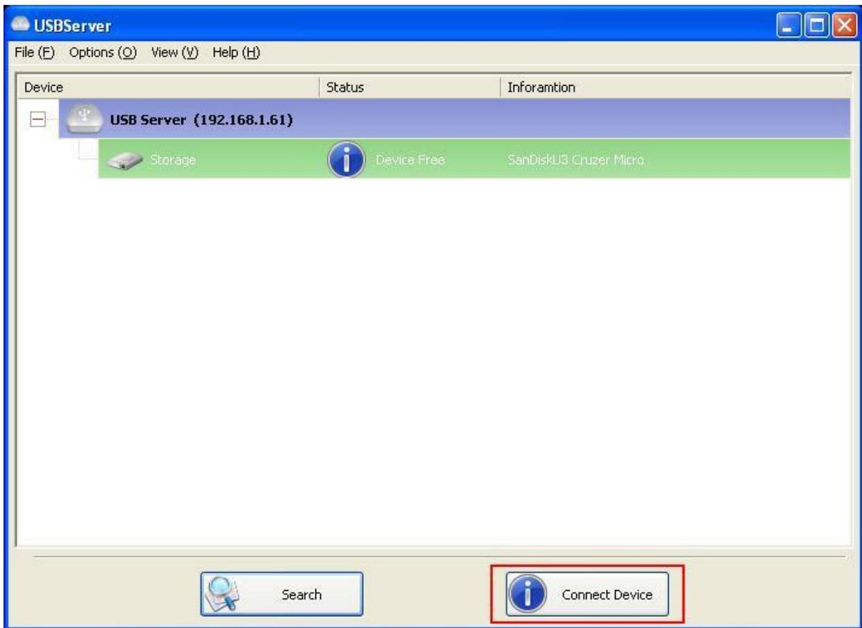
To connect to a USB device, please select it on the tree view and click on “**Connect Device**” button or double-click on it. This process might take a few seconds up to a minute, depending on the complexity of the device. **Then you can operate a connected USB device as if it were connected to your PC’s USB port directly.**
