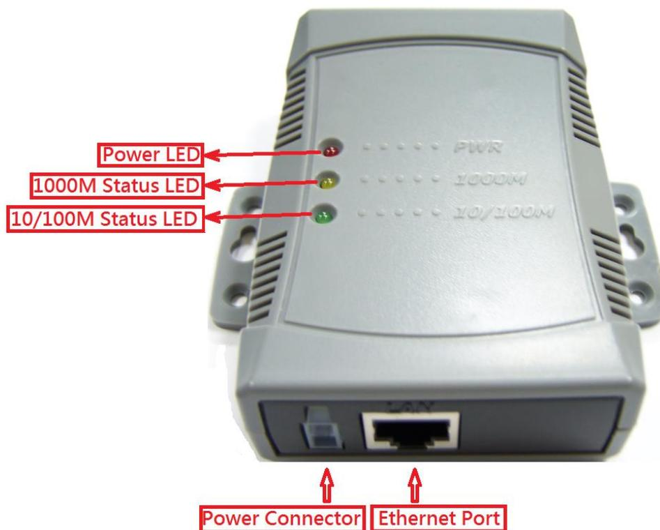
Once the Ethernet cable is connected, connect the other end of the cable to your network. This can be a free Ethernet port on your DSL router, Ethernet Hub/Switch, or an 802.11n router/ base station.
