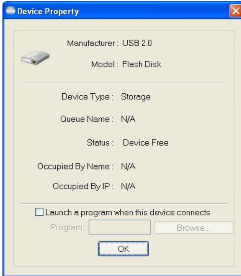
“**Device Property**” dialog box displays information of the USB device. If the device is occupied, it also displays the occupying PC name and the IP of the PC occupying it.
