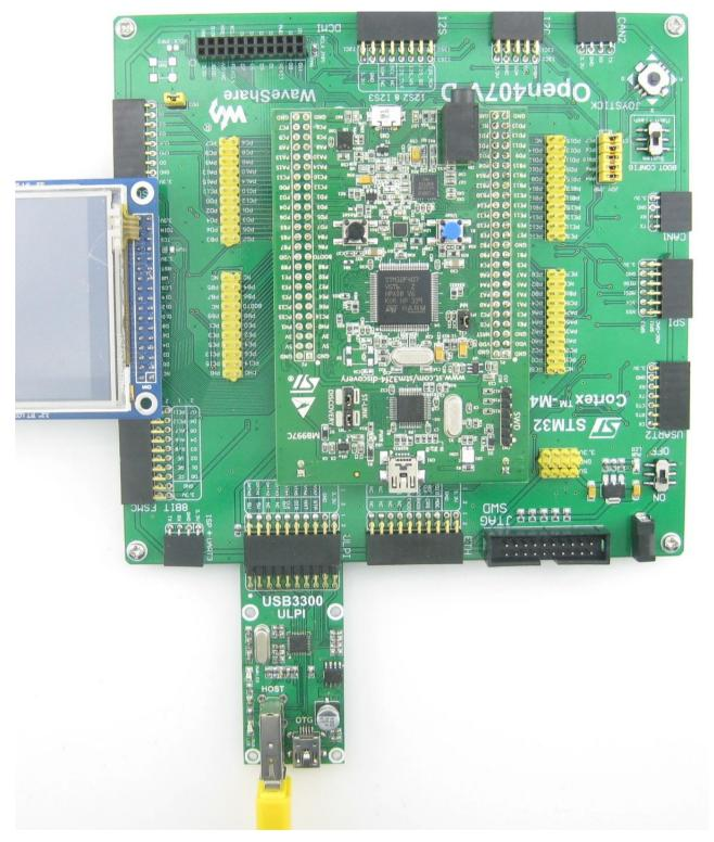
Message/info will be displayed on the LCD; the example code will place a TXT file into the USB Flash Drive, list
