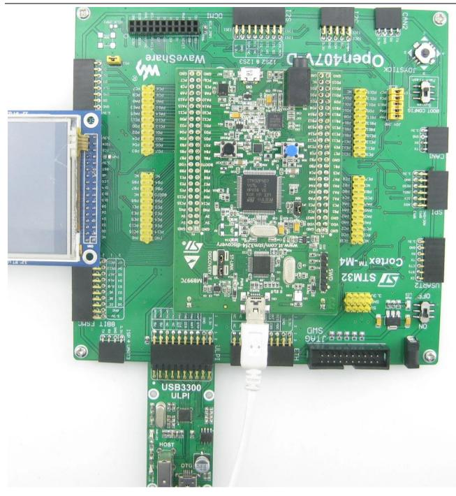
Message/info will be displayed on the LCD, and JOYSTICK can be used for simulating the mouse and controlling
