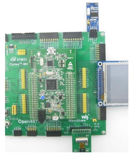
Images acquired from the camera will be displayed on the LCD.
