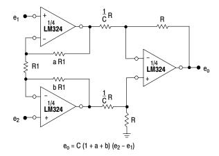
Figure 12. High Impedance Differential Amplifier
