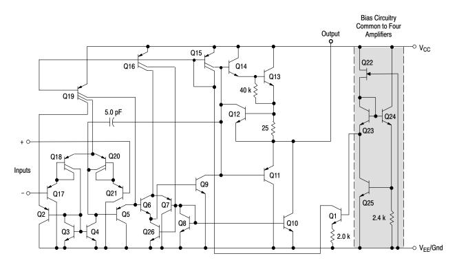
Figure 1. Representative Circuit Diagram (One–Fourth of Circuit Shown)
