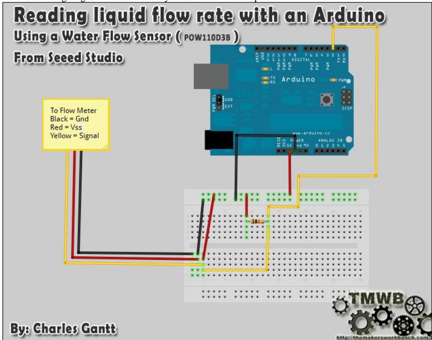
Once you have it wired up you will need to upload the following code to your Seeduino. Once it is uploaded and you have some fluid flowing through the Water Flow Sensor, you can open the serial monitor and it will display the flow rate, refreshing every second.
