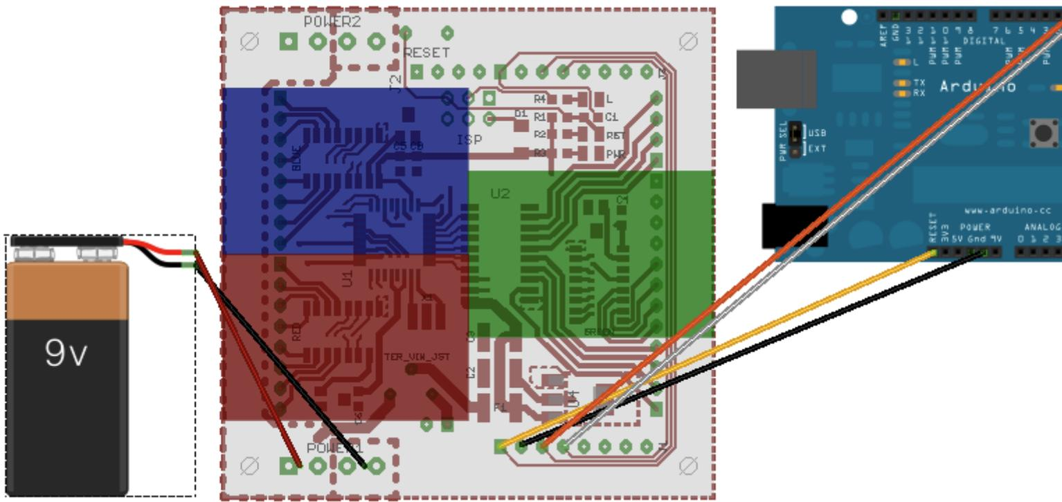
We use an external power source, however you could also use the 5V from the Arduino.
