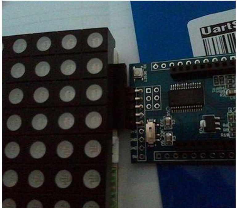
If you connect the UartSBee to the USB bus, it should register a new serial port. Now simply upload your firmware using the new serial port.
