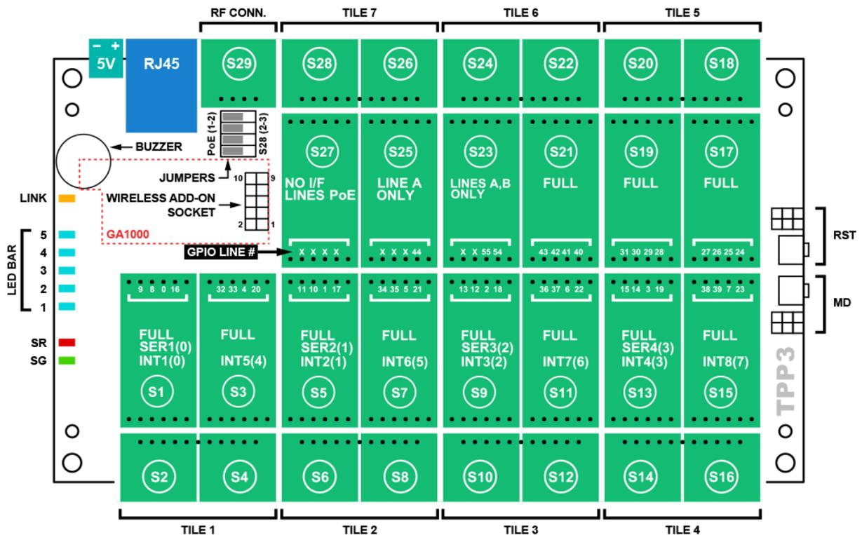
The TPP3 board features 14 x "M" and (14+1) x "C" sockets.
