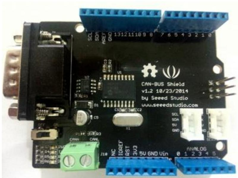
CAN-BUS is a common industrial bus because of its long travel distance, medium communication speed and high reliability. It is commonly found on modern machine tools and as an automotive diagnostic bus. This CAN-BUS Shield adopts MCP2515 CAN Bus controller with SPI interface and MCP2551 CAN transceiver to give your Arduino/Seeduino CAN-BUS capability. With an OBD-II converter cable added on and the OBD-II library imported, you are ready to build an onboard diagnostic device or data logger.
