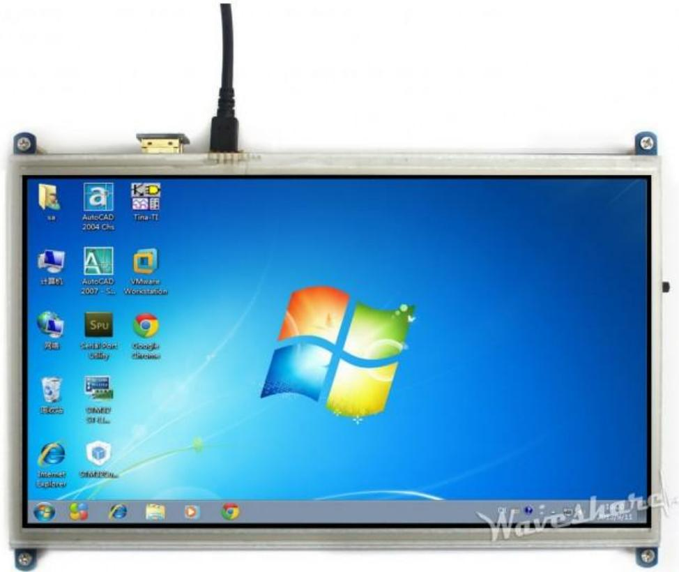
10.1inch Resistive Touch Screen LCD, HDMI interface, Designed for Raspberry Pi
